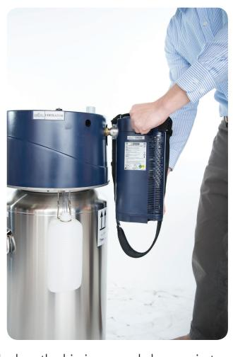
The unit is full when the hissing sound changes in tone and a dense, white vapor is seen coming from under the shroud of the reservoir. When this is observed, close the vent valve by raising its lever.
