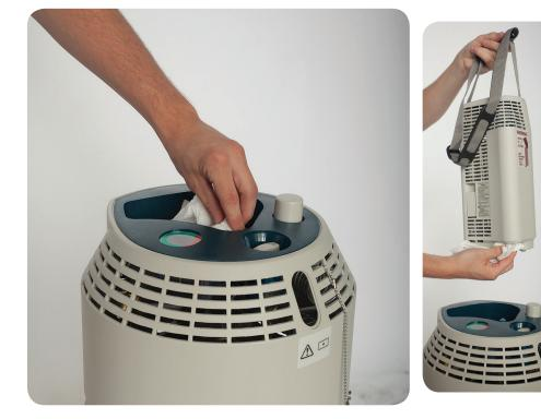
Clean the reservoir and portable unit fill connections to remove moisture and other contaminants with a lint free cloth. Do not disturb or depress the poppet on the reservoir or portable while drying the fill connectors. Also, be sure to keep the portable in the upright position at all times while wiping its fill connector.
