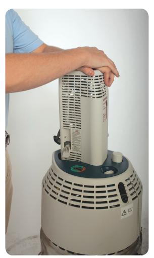
The unit is full when the hissing sound changes in tone and a dense, white vapor is seen coming from under the shroud of the reservoir. When this is observed, close the vent valve by raising its lever. 6.
