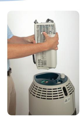
Position the portable unit above the reservoir's Quick Disconnect Valve and align it with the indentation on top of the reservoir. Press down on top of the portable unit to engage with the reservoir's Quick Disconnect Valve. Once the portable unit is engaged with the reservoir it can be filled.
