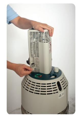
Begin filling the portable unit by simply pulling its vent valve handle into its open position while continuing to apply pressure on the portable unit to maintain its connection.
